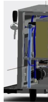
3. Remove Overflow Tube by holding collar to fitting and pulling down on the tube.
