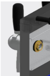
7. Secure hand on faucet(s) to be replaced and remove hex nut and o-ring from the inside. Replace faucet and hand tighten hex nut and o-ring.
