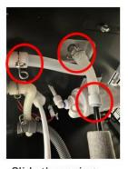
Slide the spring clamps off the stem by squeezing the ears of the clamps and disconnect the ¼" tubing. Remove the cold tank drain tube.
