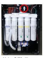
Using 5/8" silicone tubing, drain the cold tank completely into a bucket by opening the cold tank drain valve circled in RED. The tank will not refill as we disconnected the cold tank solenoid.
